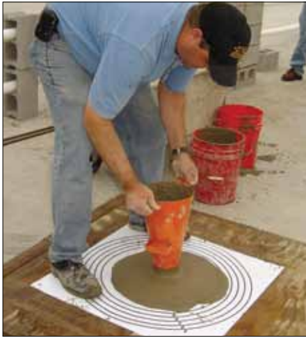
SCG Slump-Flow test targets a 20" (508 mm) spread in 2 - 5 seconds.
